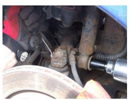
8. The damper is now hanging from the top fixing only, and best access to this is achieved by unclipping the electrical plug connections to the horns and then removing them and their brackets from the cars chassis leg.
