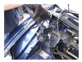
Damper removal will require the top shaft of the damper being held whilst the nut is loosened with a spanner. Once the nut is loose take hold of the damper body with your now spare hand to prevent the damper dropping out when the nut is spun off. Remove the upper washers and rubber bush.
