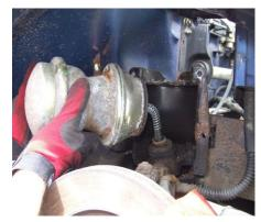
11. Retain the spacer washer that sits over the shaft of the 'knuckle' and clean off any dirt or corrosion. The spring found between the 'Knuckle' and displacer is not refitted. A light smear of copper grease will help reduce any future sticking problems. Check the rubber bump stop is in place and not been damaged or lost. If lost or damaged then a replacement will be needed.
