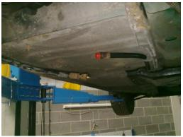
Once disconnected from these points the pipes which runs along the chassis from front to rear can be capped using the red blanking caps (supplied in the kit).
