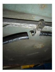
Once cut lower the pipes which were connected at the front and gentle pull the Hydragas pipe through
