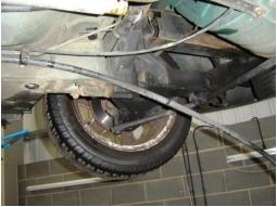
The pipes should remove freely from underneath the car.
