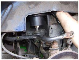
23. Follow the same set up process as described in step 13, noting that the rear springs are higher rated and so the pre-tensioning does make this much stiffer to turn.
