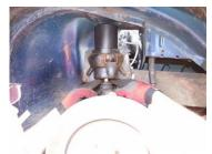
13. Once fitted in place, Using a felt pen or similar mark the front flat of the hexagon, wind out the hexagon adjuster from the SUPLEX suspension unit by 18 turns. Fit the locking ring to the threaded adjuster but do not tighten.
