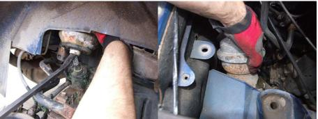
22. Select a SUPLEX rear suspension unit and fit this in from the wheel arch and 'post' it up between the body and subframe, before negotiating it into position is the same way as described in step 12.
