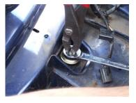
16. Refit the horns and electrical connections and then refit the plastic under wing shields.
