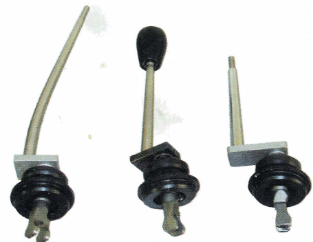
3 Selection of different gear levers used in Hi Gear five speed conversions to give the correct lever position look and look of the original gear lever
