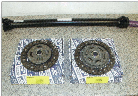
10 These five speed conversions need a hybrid clutch that usually consists of the original clutch cover that bolts to the flywheel and a driven plate that has the spline of the gearbox input shaft, with a release bearing to suit the application, all part of the kits. One off propshaft also part of the kit
