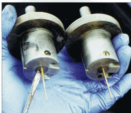
Shoulder of the needle should be flush with piston base, not proud as shown on the left hand example
