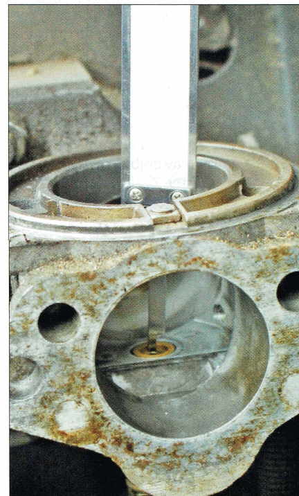
A vernier caliper is used to measure the distance between the top of the bridge area of the carburettor
