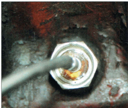
Colourtune showing red for too rich a mixture
